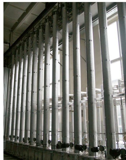
Current Manufacturing process of Lightwater (Vacuum Fractional distillation–rectification)
